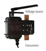
The LV-Guard 250 intelligent electronic power switch is inserted directly into the fuse block instead of the NH fuse. It permits the continuous supply of power to the low-voltage network and at the same time takes over the function of an electronic fuse. If it is tripped, a fault pattern is automatically recorded: Depending upon the equipment, TDR reflection images, current and voltage diagrams and impedance values are available to you.
